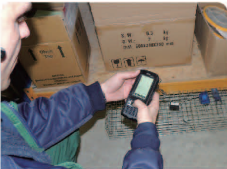
The catch boxes are equipped with a barcode and thus provide information on the kind and the intensity of the pest infestation.
