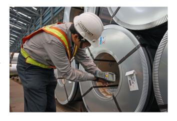
To scan bar codes on the stacked rolls while standing on the floor, 8500 mobile computers with extra-long-range lasers, which can read barcodes from over 13 meters, were chosen. Using the ergonomic pistol grip, workers use the 8500s for hours without fatigue. For warehouses storing smaller coils, CSC chose 8061 mobile computers for their handy pocket size and lower cost. With the deployment of the CipherLab 8061 and 8500 mobile computers, cycle counts are completed in half the time.
